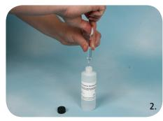
**2.** Snap off the tip of one end of the ampule using the supplied ampule breaker.
